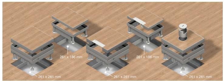
Quadrangular cartridge unit with hem, made of stainless steel, as a dummy cartridge unit, cable outlet cartridge unit and tube cartridge unit for the installation into screed and hollow floors. For 12/22/32/42 mm parquet and stone covers and linoleum in combination with rigid foam lid insert. Can be levelled from 65 to 315 mm.
