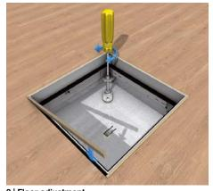
**3** | Floor adjustment Align the installation frame flush to the level of the finished floor with the four levelling screws. Seal the expansion joint all around with a suitable sealing compound.
