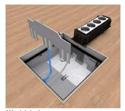
**4** | Lock-in leads Mount both lock-in leads with two screws each on the side of the frame. Create grounding connection between levelling device and floor box. When using a coupler plug H = 35 mm, comply with the minimum installation depth Hmin = 95 mm.
