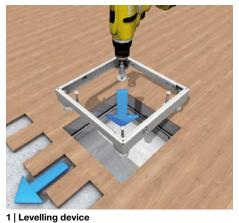
For parquet or stone floors insert the levelling device into the floor opening. Fasten the four levelling bases with nail plugs.
