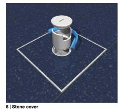
For wet maintenance floor covers such as stone covers, only a tube cartridge unit may be used. However, the floor cover depth must be considered. Insert the replaceable cartridge into the frame. The tube can be screwed. Observe the potential equalization.
