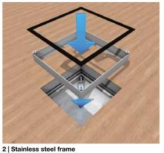
Screw the stainless steel frame to the levelling device with four screws. Glue rubber seal in place. Make the grounding connection between levelling device and floor box. A regular maintenance and cleaning of the seals is
