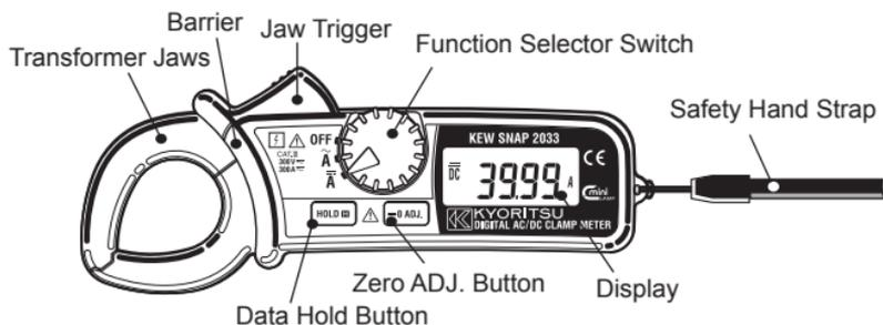
Barrier is a part providing protection against electrical shock and ensuring the minimum required air and creepage distances.
