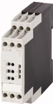
**Overcurrent and undercurrent monitor, Current measuring range: 0.3 - 1.5 A, 1 - 5 A, 3 - 15 A, Supply voltage: 24 - 240 V AC, 50/60 Hz, 24 - 240 V DC**
